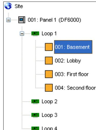
To add a device, select the detection zone the device will occupy. This can be found on the panel loop shown in the site overview on the left hand side of the screen.
