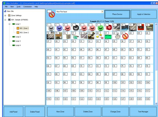
To add multiple devices of the same type at the same time, select the device type from the drop down list of types, select the addresses required and then select the **Apply to Selection**.
