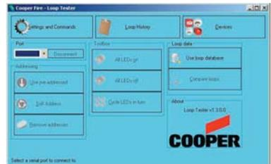
Upon successful connection to the loop tester hardware, you will be informed in the status bar and the features for interfacing with the loop will be enabled.
